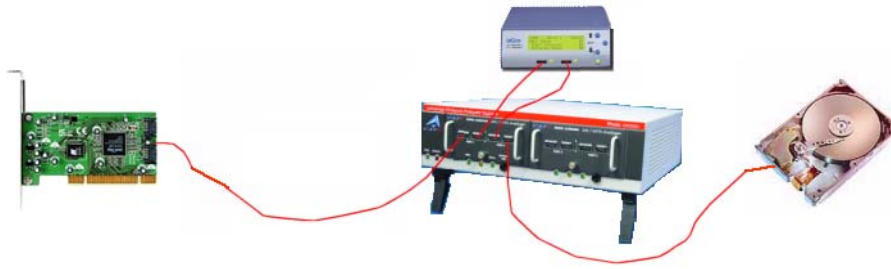
Figure 3.15 Connection With Analyzer: Two-Channel Configuration
