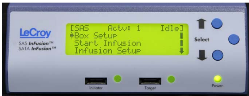
Figure 2.1 SASInFusion Front Panel
