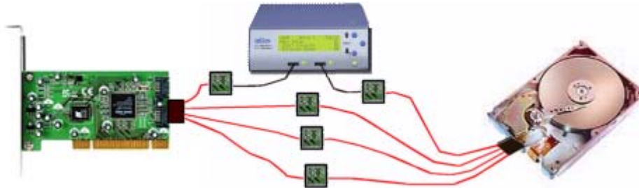
Figure 3.16 Multiple Connections Using "Octopus" Cables
