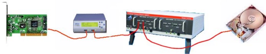
Figure 3.14 Connection with Analyzer: One-Channel Configuration
