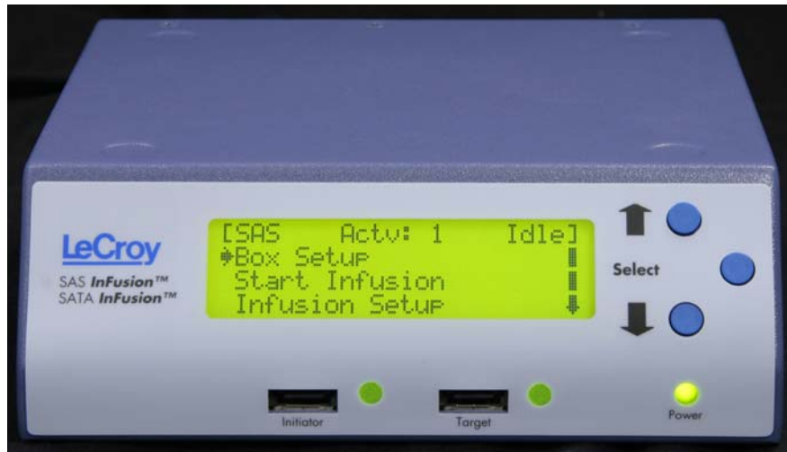
Figure 6.1 SASInFusion LCD Panel
